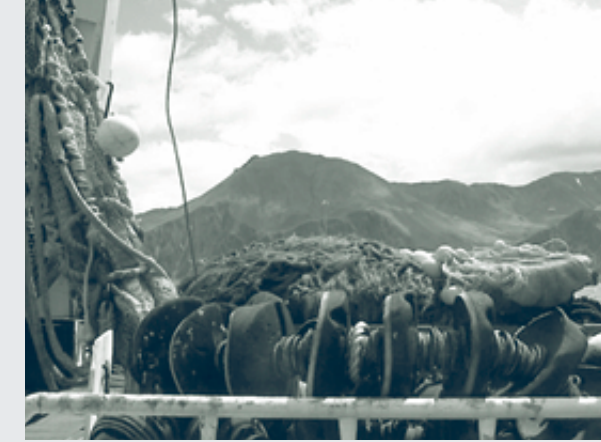
Roller gear (pictured here) and rockhopper gear span the base of bottom trawl nets, allowing the nets to be dragged through and over rough seafloor habitats. Photo: AMCC
